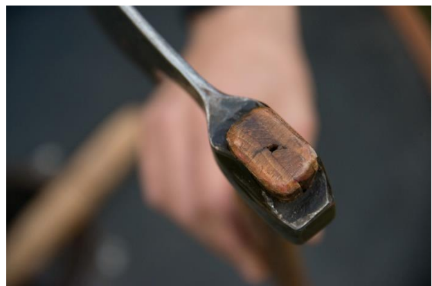
Image 8.0 (Left) Shows a bearded axe (Type D) Note that the lugs are flat against the woode haft and not proud of the wood. Note that there is only a small amount of wood protruding above the top of the socket.
